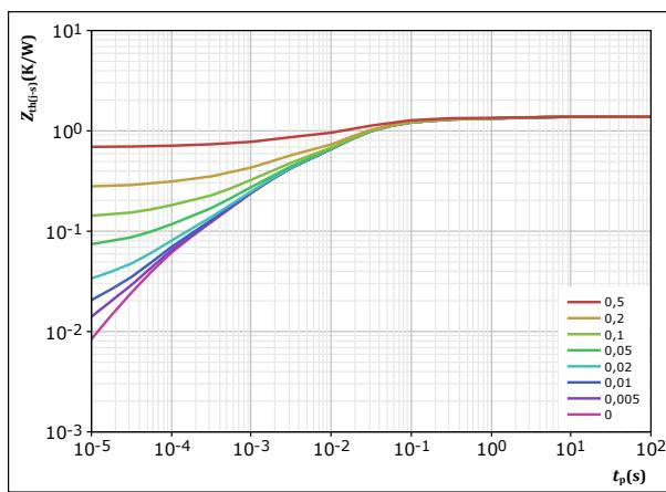
$$D = \frac{t_p}{T} \quad R_{th(j-s)} = \frac{t_p}{1,382} \quad K/W$$
