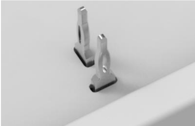
5. Figure Copper visible on Press-fit pins
